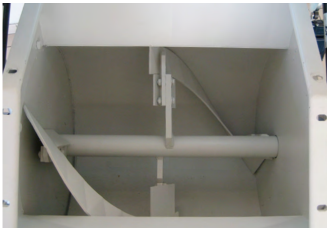
View inside with exchangeable mixing tools.
