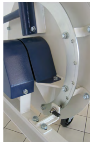
Maintenance-free bearing. Lockable slewing.
