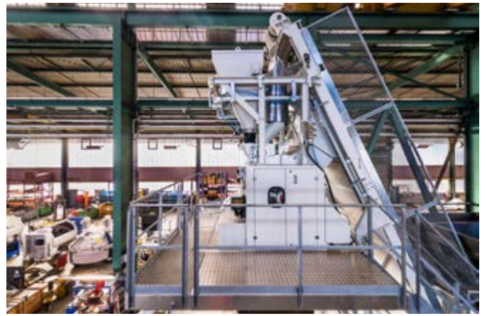
Generous service and maintenance platforms ensure best service accessibility
